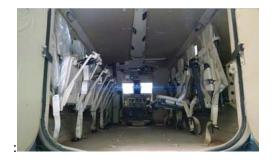
Inside up front with portable radio mounts, antenna connections, the siren/pa box, and the backup camera monitor shown
