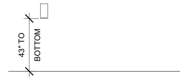
1 ACCESSORY MOUNTING DIAGRAM 1/4" = 1'-0"
