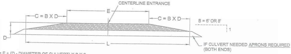
L = E + (D - DIAMETER OF CULVERT) X B X 2
