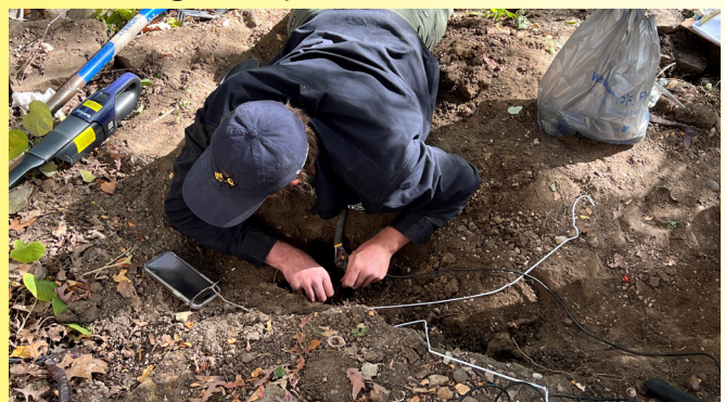
Above: Kyle Price uses an endoscope to view the network of underground tunnels. Images from the scope were streamed on his phone.
