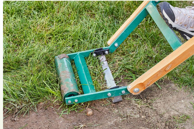
A sod-cutter removes grass.
